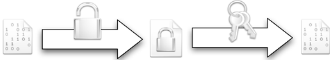
Fig. 7.5. Asymmetric key cryptography encrypts data with one “public” key. Decryption is possible only with the “private” key
