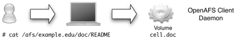
Fig. 5.2. Users request a file without any further knowledge. The AFS client retrieves the actual volume the data resides on
